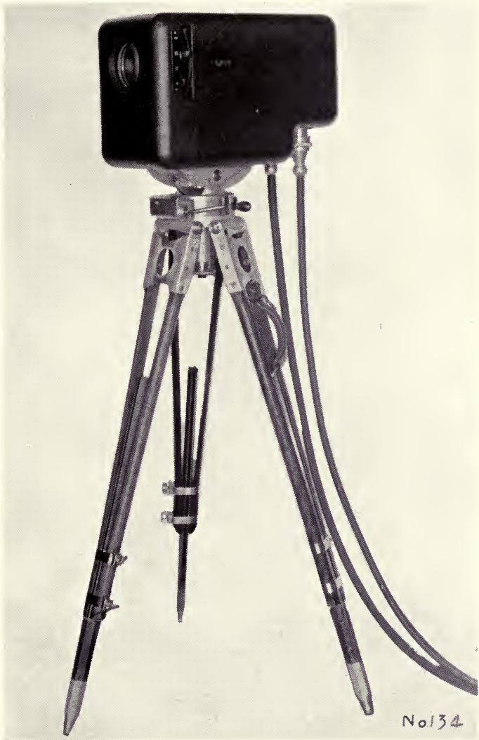
Fig. 13. The Farnsworth Pick-Up Camera complete. (Note compactness)
